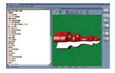
VR CNC Turning is a Virtual Reality based CNC programming software package offering full machine control and Virtual Reality simulation of CNC Lathes. Features include customisable docking toolbars, comprehensive tooling management, colour formatting of NC code & powerful NC code modification options.
