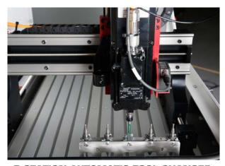
**5 STATION AUTOMATIC TOOL CHANGER** The 5 Station Automatic Tool Changer is now **supplied as standard** on the new Router 2600 ATC and Router 6600 ATC and is NOT available as an optional accessory. It comes complete with 5 SK11 Toolholders and 8 collets and offers the following benefits:
